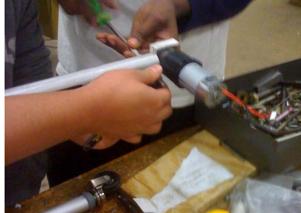
Fig 7.11: Attaching Motor Assembly to Leg
