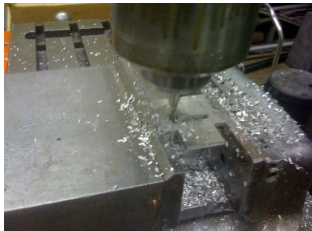
Fig 7.9: Milling Slot in Bracket
