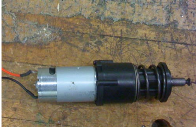
Fig. 6.3: Drive wheel Motor from Hand Drill
